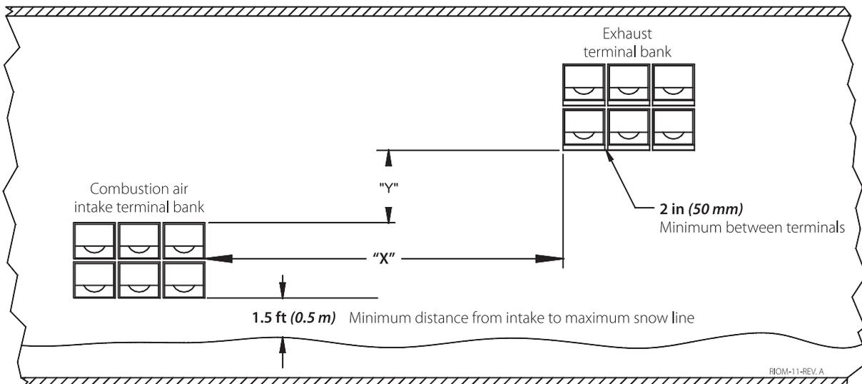
**Figure 3** Vertical Air Intake and Venting for a Direct Vent System
