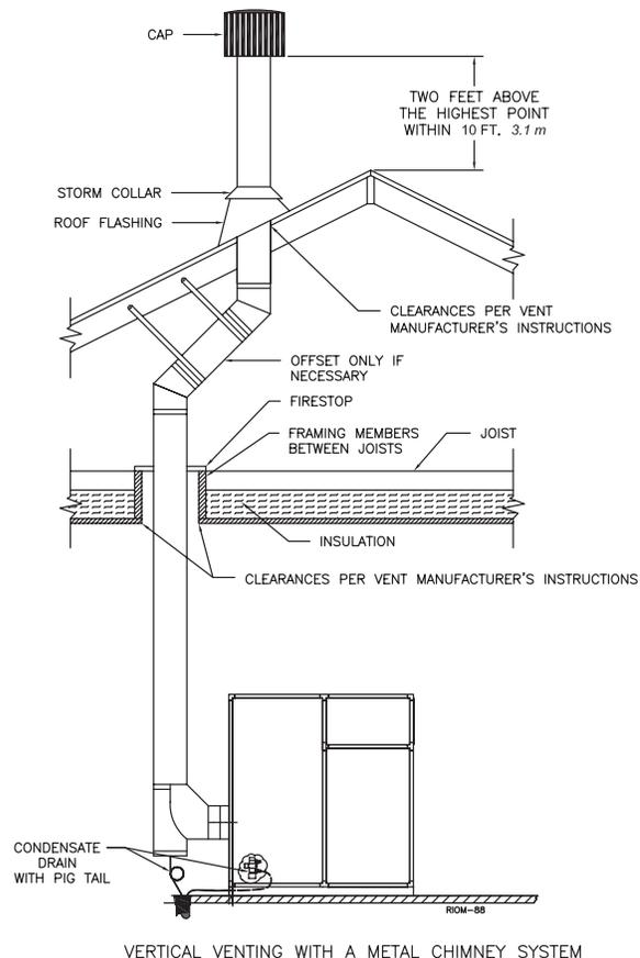
**NOTICE** Multi-story, common venting systems shall be in accordance with the National Fuel Gas Code, ANSI Z223.1/NFPA 54 and/or the CSA B149.1, Natural Gas and Propane Installation Code (Current Editions), local codes and vent manufacturer's installation instructions. Size the chimney and breeching using generally accepted engineering practices. (Consult factory for vertical heights beyond 60 ft.)
